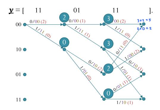
Each circled number at a node is the running (cumulative) path metric, obtained by summing branch metrics (distance) up to that node.
